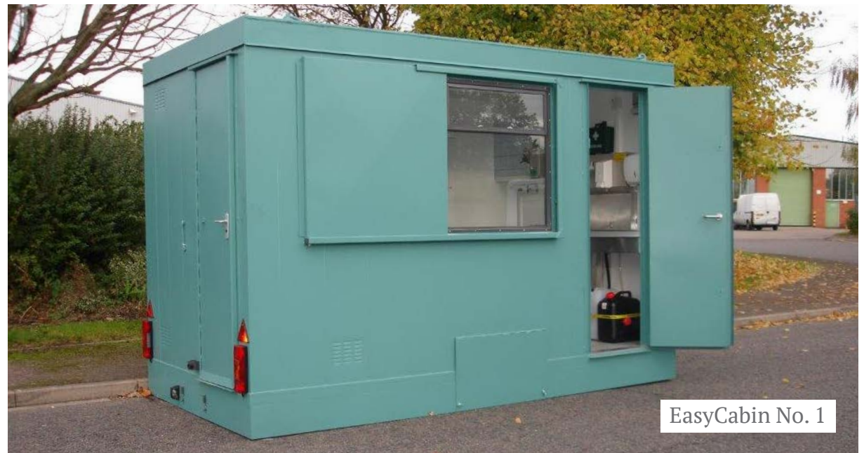
October 2005, the first AJC welfare unit with hydraulic axles. The current EasyCabin 12 design evolved from here.
